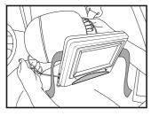
2) Tightly wrap the mounting strap around the headrest.
